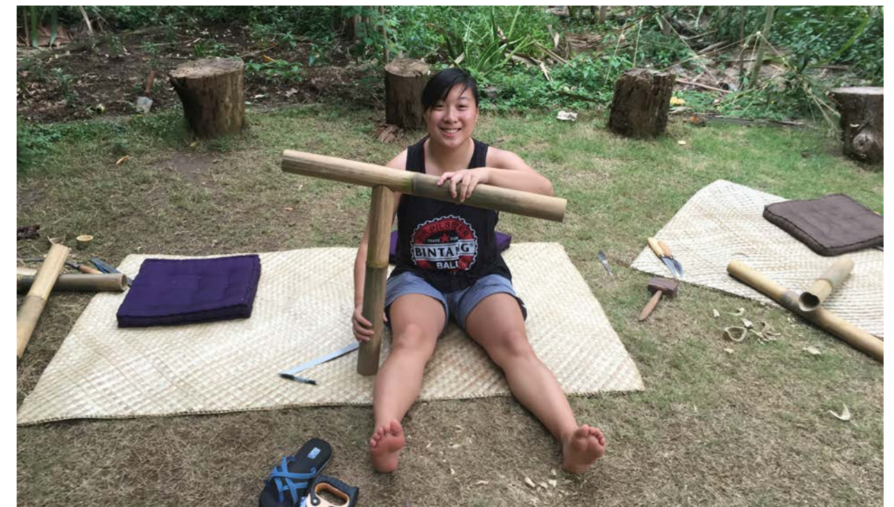
Figure 2: Wentworth Architecture and Bamboo U student Jonah He proudly displays a traditional “fish mouth” joint made with simple hand tools, Sibangkaja, Bali (Robert Cowherd CC BY-SA).
