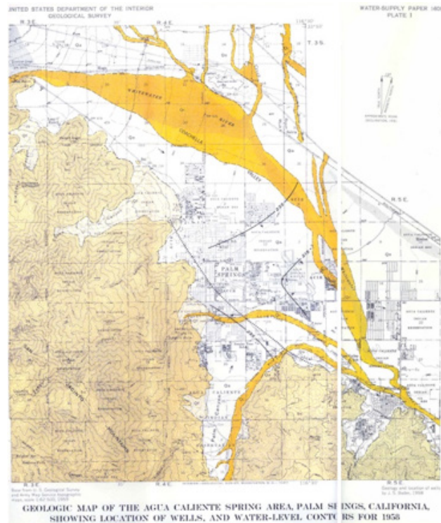
Figure 6: "Geologic map of the Agua Caliente spring area, Palm Springs, California, showing location of wells, and water-level contours for 1958." L. C. Dutcher and J. S. Bader, Geology and Hydrology of Agua Caliente Spring, Palm Springs, California . Washington, U.S. Govt. Print. Off., 1961.
